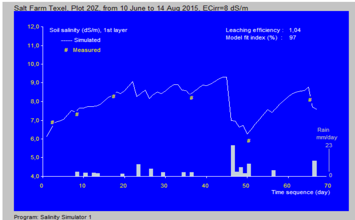
Figure 12. Overview of the measured and modelled root zone salinity during the season of 2015, data shown of a plot irrigated with water having a salinity of 8 dS/m. After 20 days the soil salinity in the first layer (40 cm) of the root zone reaches the value of 8 dS/m to equalize that with the salt concentration of the irrigation water. Rain showers (represented by white bars) caused a reduction of the soil salinity, especially around day 50.
